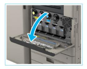
2 Remove the dust proof glass cleaner from the rear side of the front cover of the main unit.
