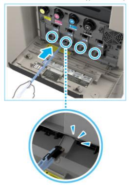
4 When you have finished cleaning the dust proof glass, gently push the dust proof glass cleaner back onto the rear side of the front cover of the main unit.
