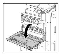
Release the Waste Toner Box Lock Lever, and then remove the Waste Toner Box.
