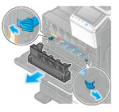
**3.** Remove the Printhead Cleaner from the Lower Front Door or Front Door of this machine.
