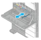
**3.** Securely press the Charger Cleaner, and close the Lower Front Door or Front Door of the machine.
