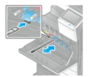
**5.** Mount the Printhead Cleaner onto the Lower Front Door or Front Door of this machine.
