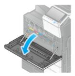
2. Release the Waste Toner Box Lock Lever, then remove the Waste Toner Box.
