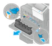
3. Remove the Printhead Cleaner from the Lower Front Door or Front Door of this machine.
